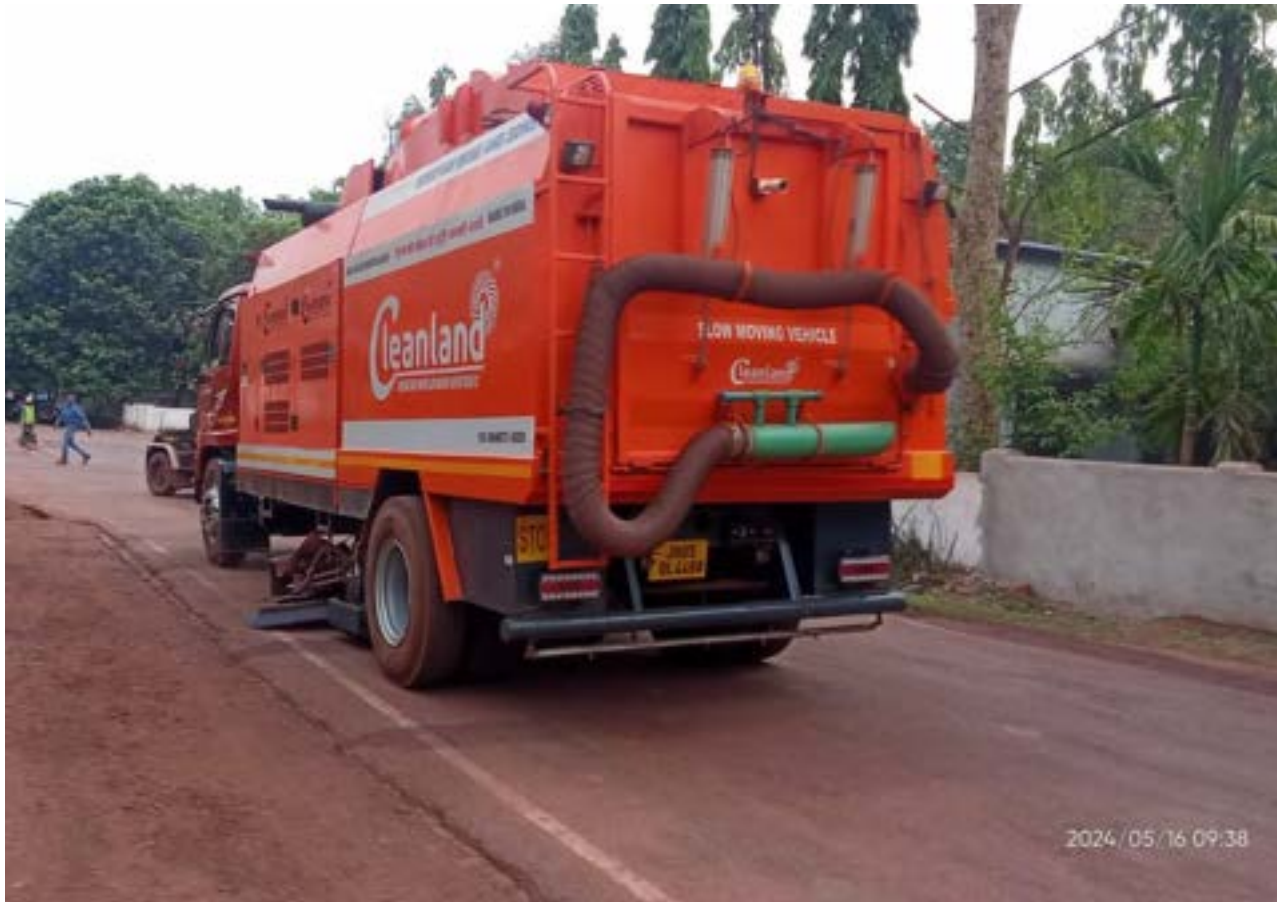
Vacuum Sweeping Machine in Operation
