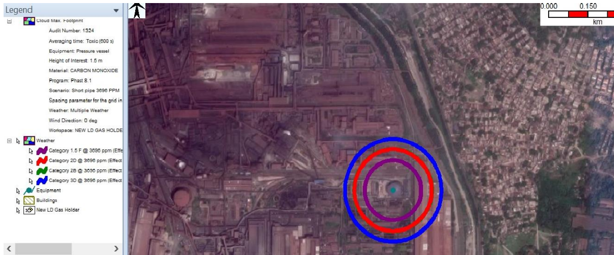
Figure 9.3: Foot prints of CO gas for the catastrophic release from LD gas holder (60000 m 3 )
