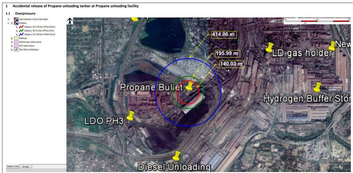
Figure 9.12: Explosion Overpressure for the release of propane unloading tanker
