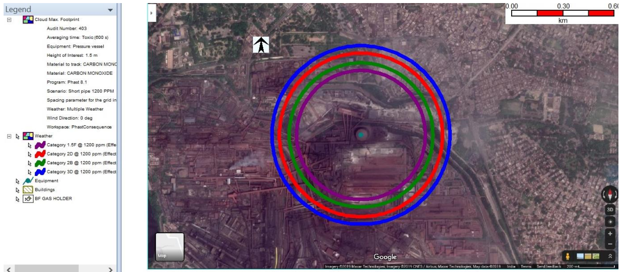
Figure 9.1b : Foot prints of CO gas due to catastrophic release of BF gas Holder (1200 PPM)
