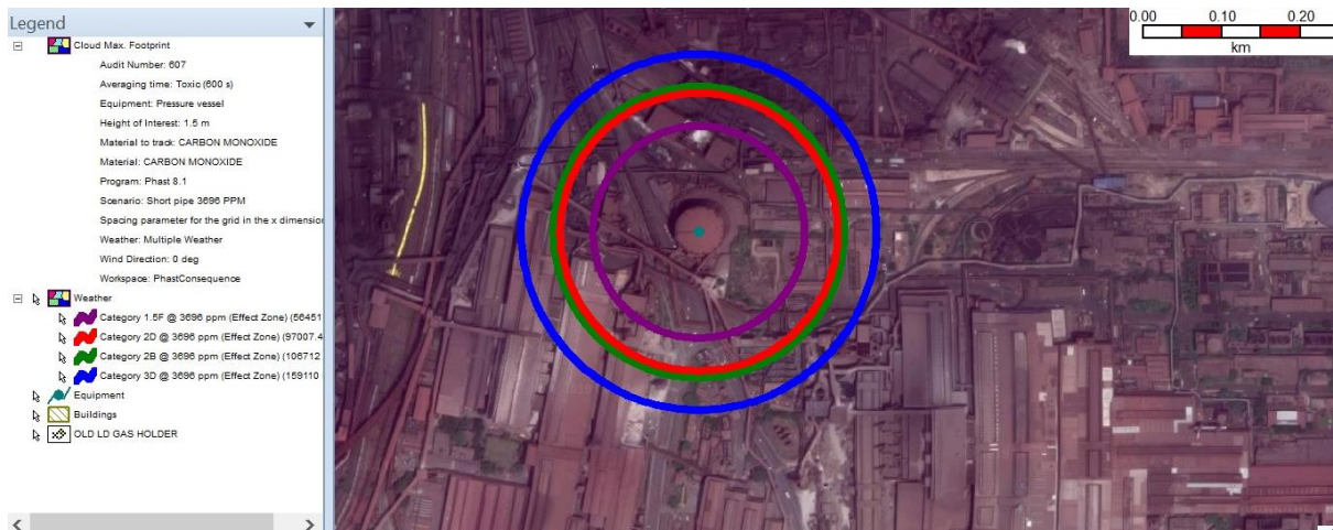
Figure 9.2: Foot prints of CO gas for the catastrophic release from LD gas holder (100000 m 3 )
