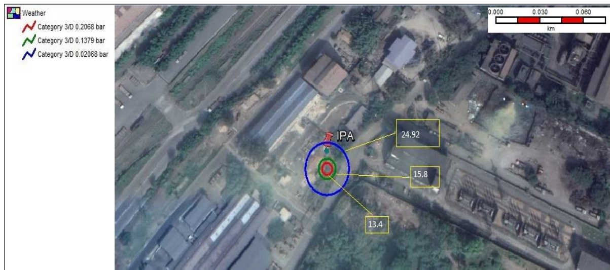
Figure 9.19: Explosion Overpressure for IPA Tank Catastrophic Rupture
