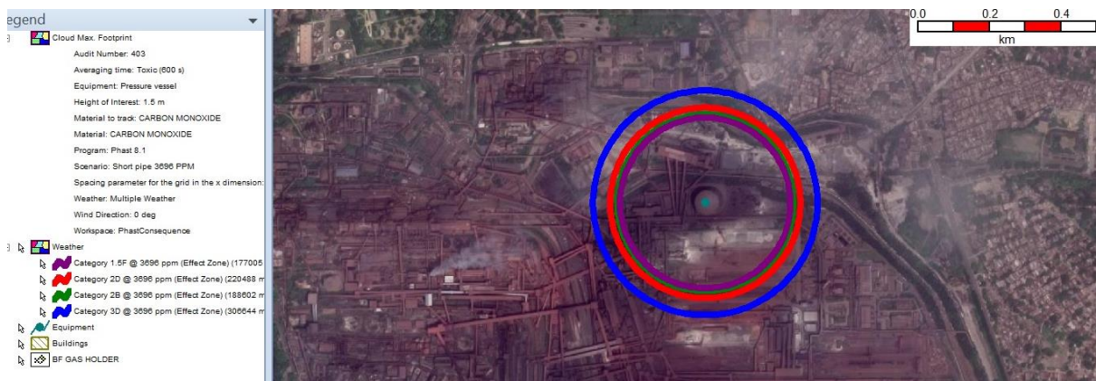
Figure 9.1a : Foot prints of CO gas due to catastrophic release of BF gas Holder (3696 PPM)
