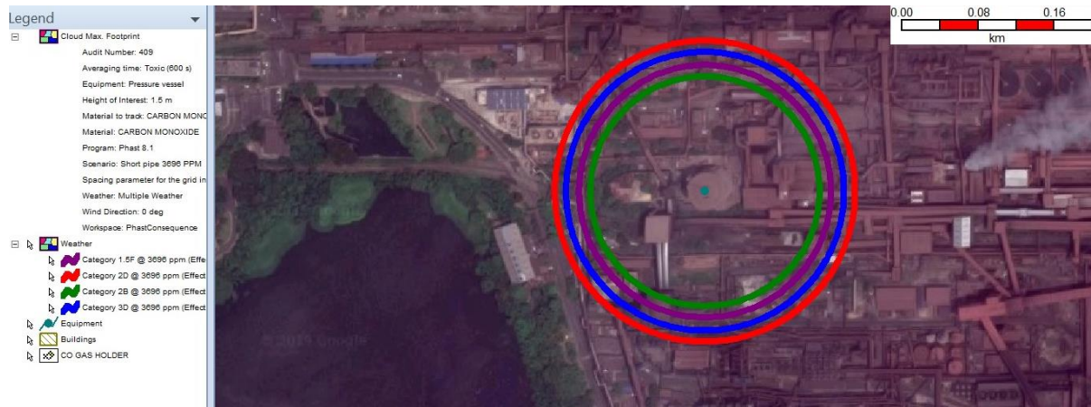
Figure 9.4a : Foot prints of CO gas due to catastrophic release of CO gas Holder
