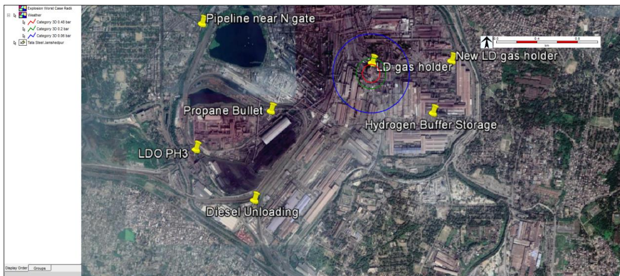
Figure 9.7: Explosion Overpressure for the release of CO from LD Gas holder (100000 m 3 )
