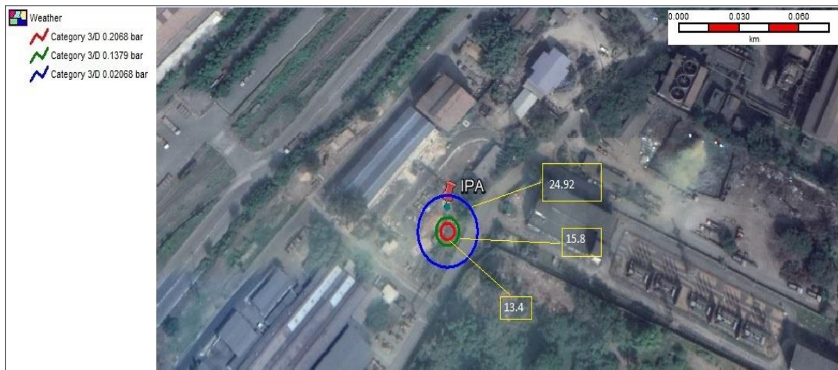
Figure 9.19: Explosion Overpressure for IPA Tank Catastrophic Rupture
