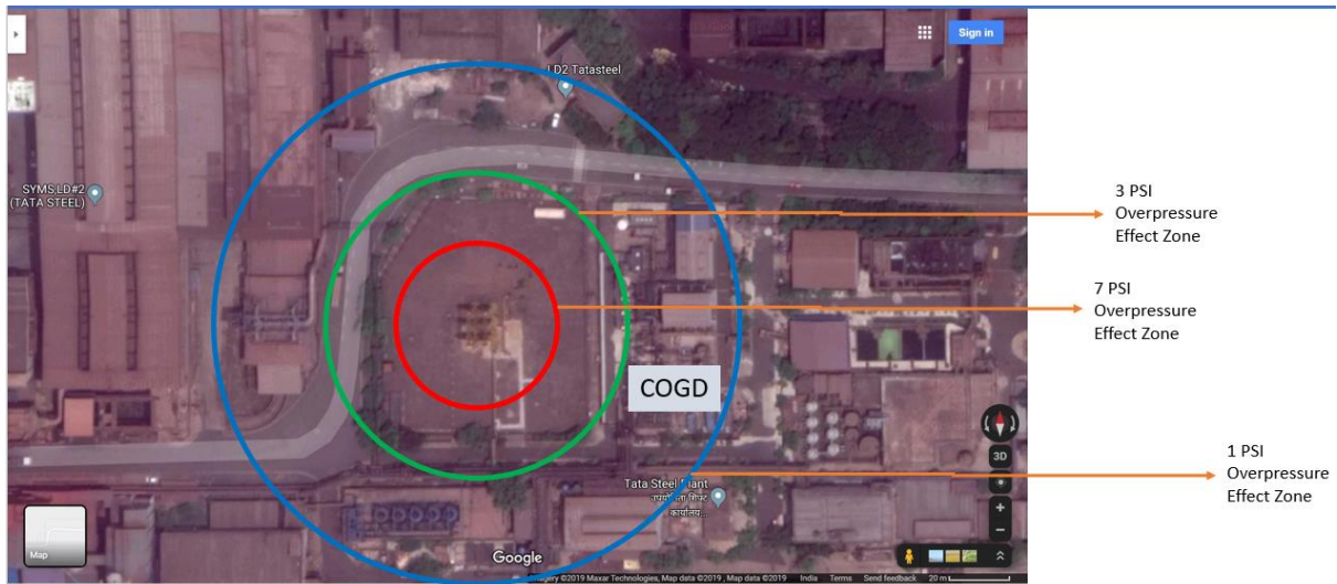
Figure 9.20: Explosion Overpressure for Hydrogen buffer tank Catastrophic Rupture
