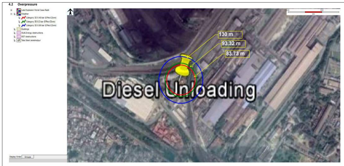
Figure 9.16: Explosion Overpressure for the release of Diesel unloading tanker
