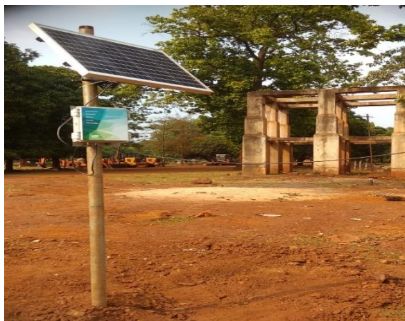
Piezometers installed for Ground water level monitoring.
