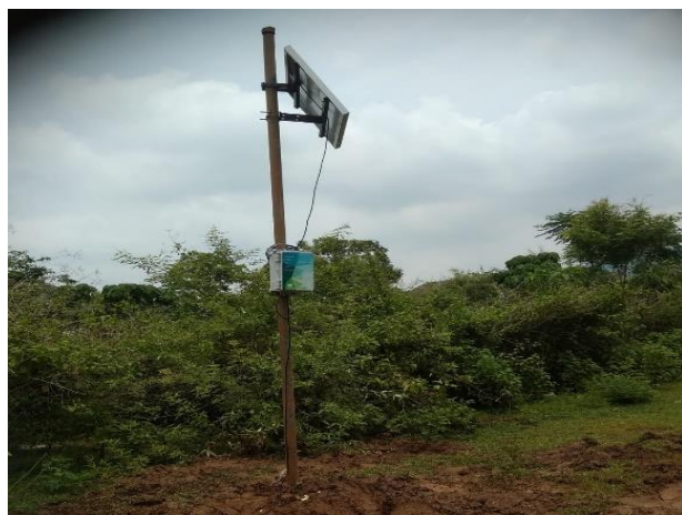
Piezometers installed for Ground water level monitoring.
