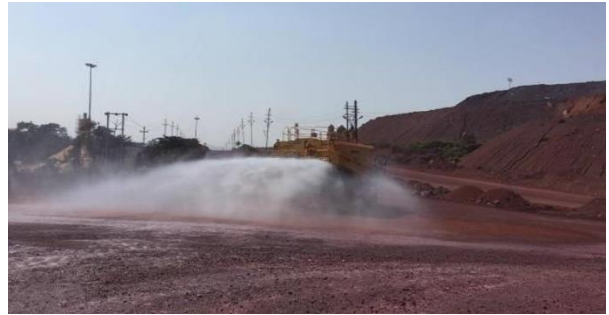
Use of mobile water tanker for water sprinkling on haul roads
