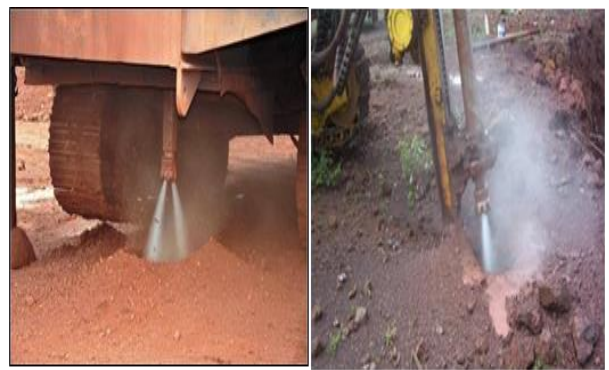
Wet drilling to control dust emission
