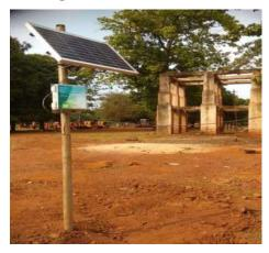
Piezometers installed for Ground water level monitoring
