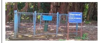
Piezometric bore well at Katamati Iron Mine
