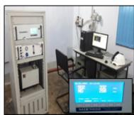
Continuous Emission Monitoring for Power House for PM, Sox & NOx data
