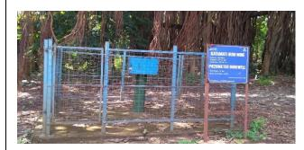
Piezometric bore well at Katamati Iron Mine
