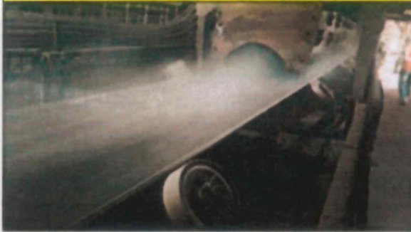
Use of Dry fog system at all transfer points in plants
