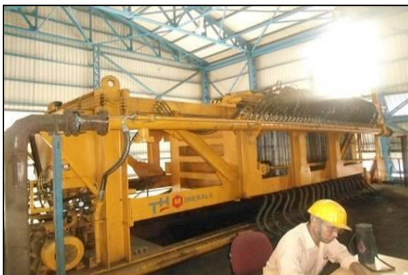
Mechanical tailings de-watering system
