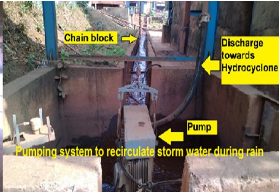
Tailing Dewatering Plant and Water Recirculation Arrangement
