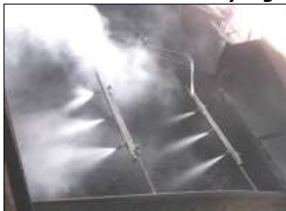
Dry fog dust suppression system in crushing units
