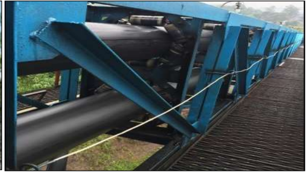
Pipe Conveyor for material transport
