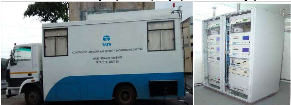
Continuous Ambient Air Quality machine (CAAQMS) for data monitoring system
