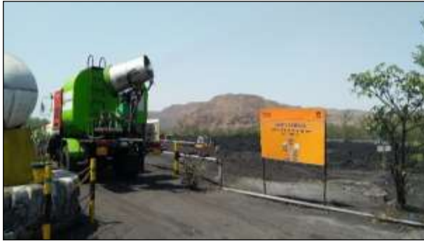
Water Mist Canon in coal stacking area
