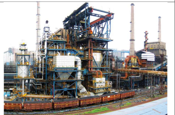
Waste Heat Recovery in Coke Dry Quenching
