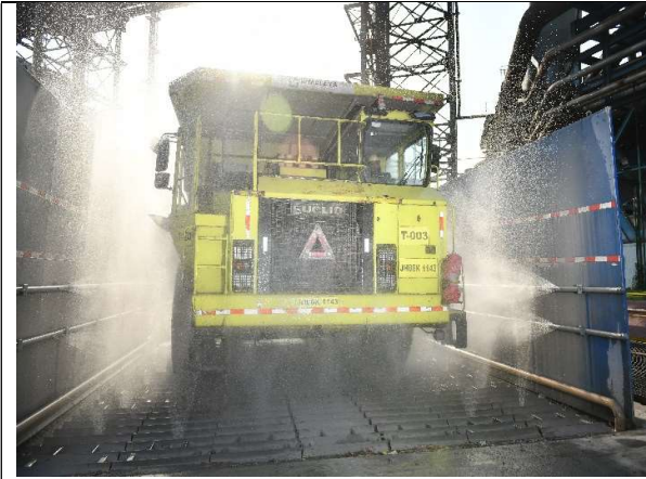
Tyre Washing Facility (TWF)
