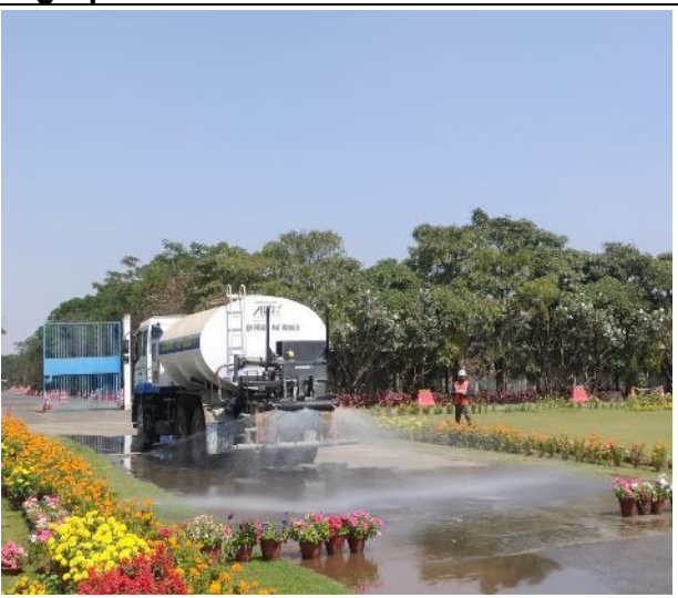
Mist type high jet water sprinkler for dust suppression
