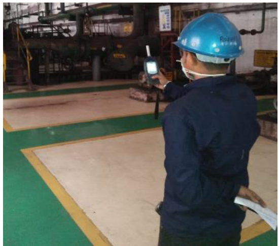
Work Zone Noise Monitoring
