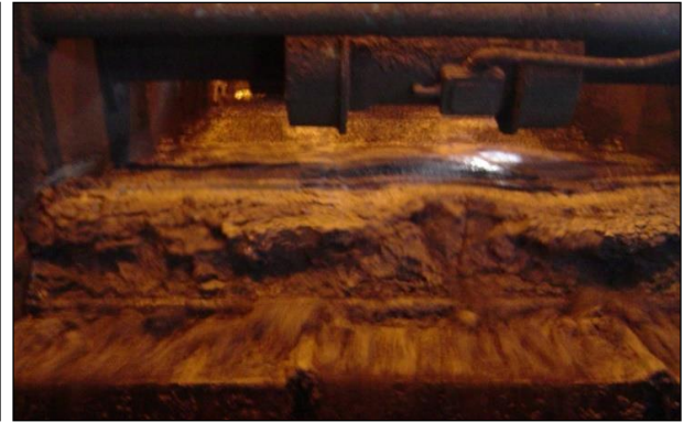
Output of HFC at tailing dewatering plant
