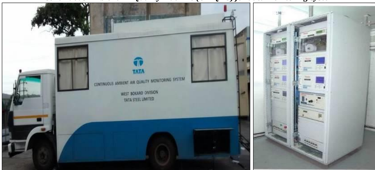
Continuous Ambient Air Quality machine (CAAQMS) for data monitoring system
