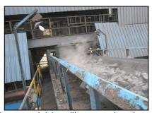
More than 2.5 Kilometers of the road inside the material handling area has been paved to reduce the dust generation. The total coal yard (area of 25000 sq. Mt.) has also been concreted in order to prevent the dust generation.
