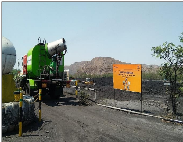
Water Mist Canon in coal stacking area
