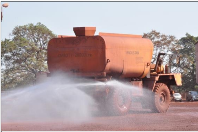
Mobile Water Sprinkling
