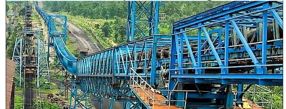
Long Pipe Conveyor at West Bokaro to reduce environmental footprint in coal logistics
