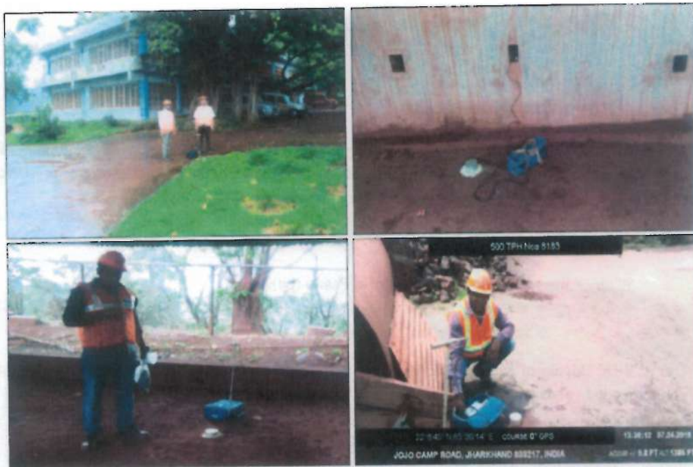
Photograph 2. Monitoring of vibration at different locations of the Noamundi Iron mine of Tata Steel Ltd.
