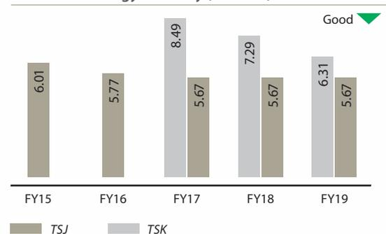
\* Coke rate means kilograms of coke used to produce 1 tonne of liquid iron in blast furnace
