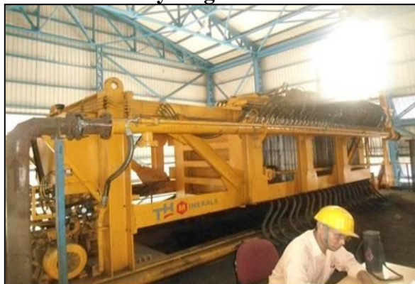
Mechanical tailings de-watering system
