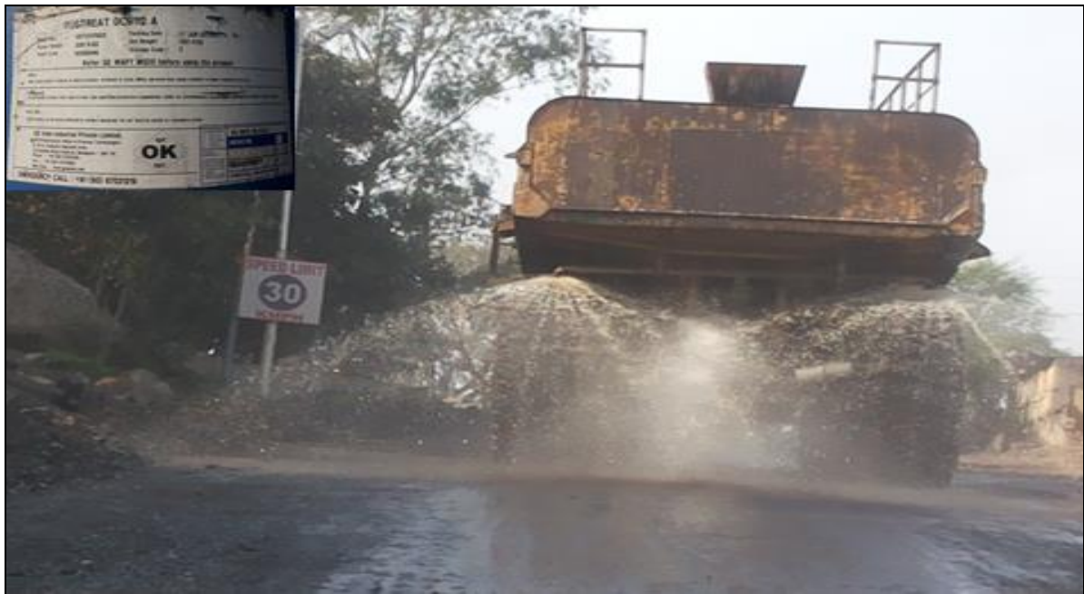
Pressurized water spraying in mines area with chemical dosing
