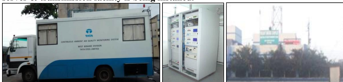
Continuous Ambient Air Quality machine (CAAQMS) for data monitoring system
