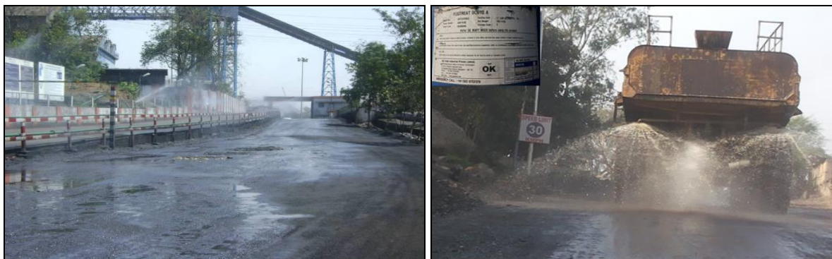
Fixed and mobile water suppression system
