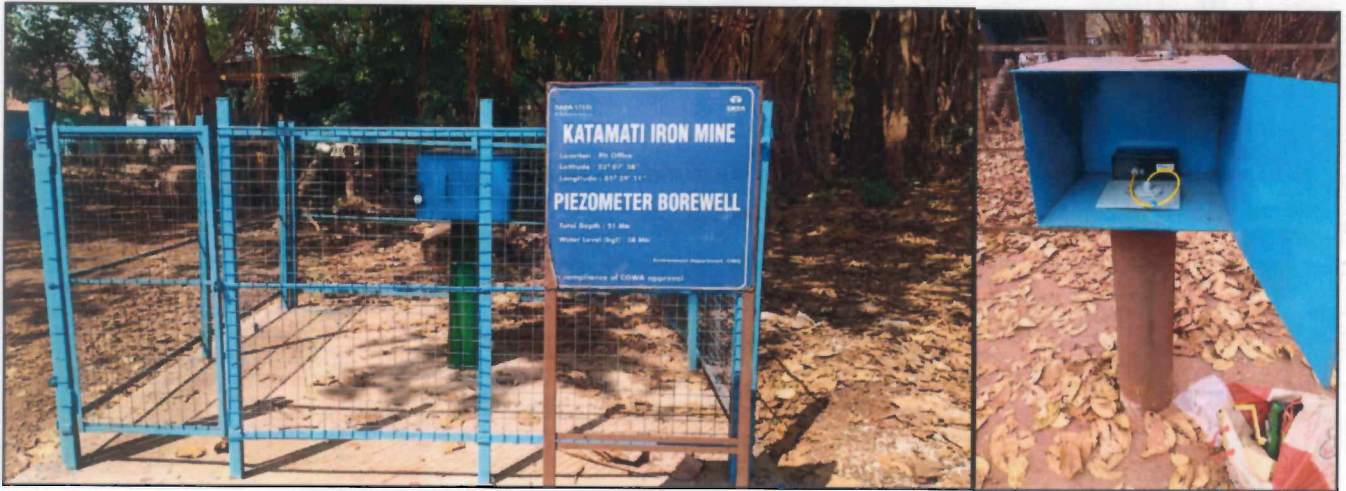
Piezometric borewell installed at Mine Office site, Katamati Mine
