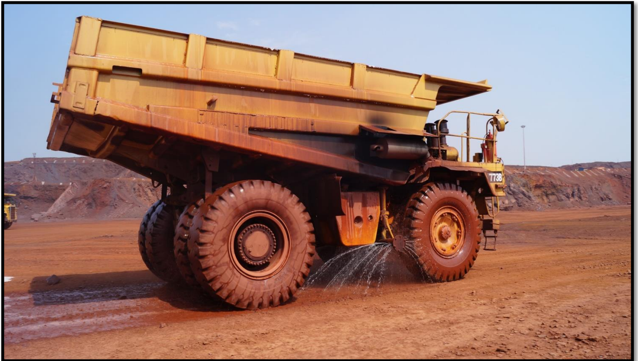
Mobile Water Sprinkling
