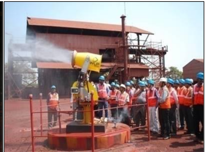
Water Mist System in Plant
