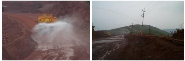
Mobile & Fixed water sprinklers in Noamundi mines
