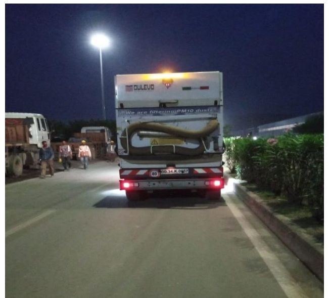
Mechanised road dust sweeping
