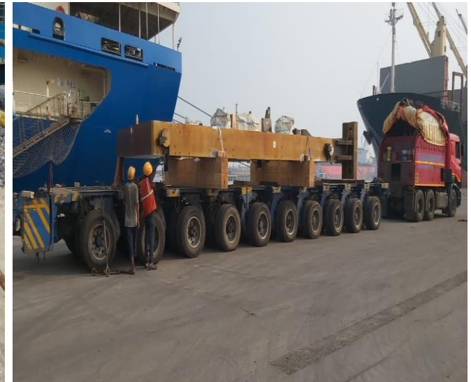
4 Mill Housings received
